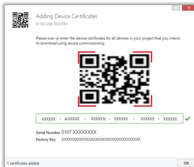
Fig. 7: Interra KNX Secure IP Router Adding Device Certificates
